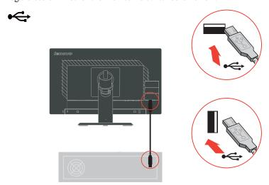
8. Connect one end of the USB cable to the USB upstream terminal on the side of the monitor, and connect the other end of the USB cable to an appropriate USB port on your device.
